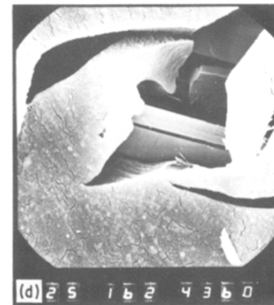
Figure 8 A sequence of scanning electron fractographs of the side of the specimen showing details of a delamination failure mode.
